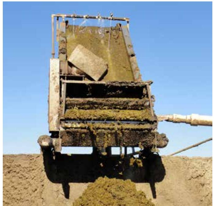
Manure fibres, sand and gravel, waste feed and other bits and pieces are all responsible for causing trouble in effluent systems. It can be helpful to separate some of these solids from the effluent stream to prevent them wearing out pumps and equipment, and blocking irrigation systems. Separating solids will mean the pond needs to be de-sludged less often, or may prolong the life of an otherwise overloaded pond.
