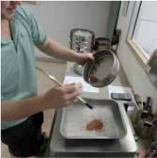
**A Particle-size Analysis,** or how much clay, silt and sand there is in the soil. The clay content is required for the pond to seal.
