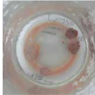
**The Emerson Aggregate Test,** to see how dispersive or prone to erosion the soil is.
