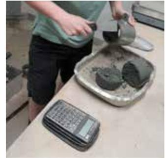
**The Proctor Compaction Test,** to find the range of moisture contents over which the required level of compaction can be achieved.
