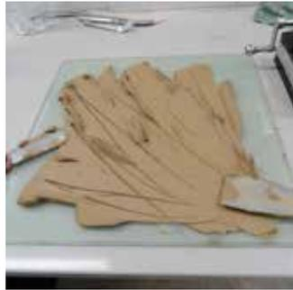
**The Atterberg Test,** determines the clay's plasticity.
