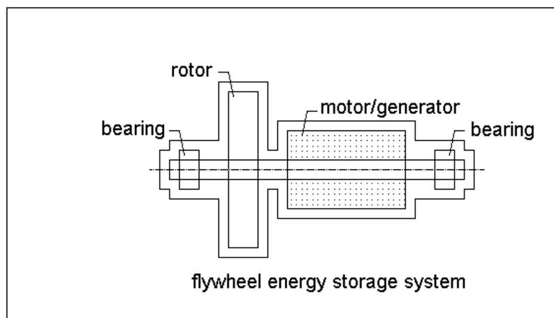
Figure 4.5: Cross-section of a Flywheel
